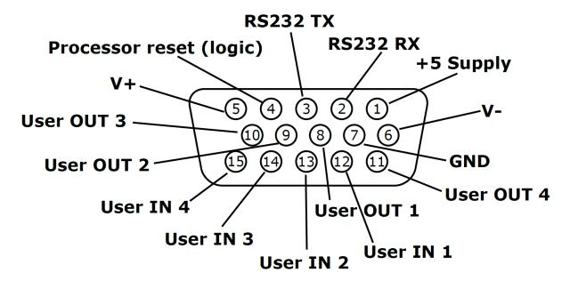
Figure B.1 DE-15 GPIO Port Functions
