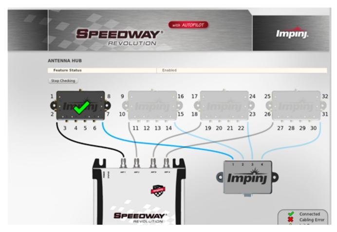
Figure D.4 One Antenna Hub Detected
