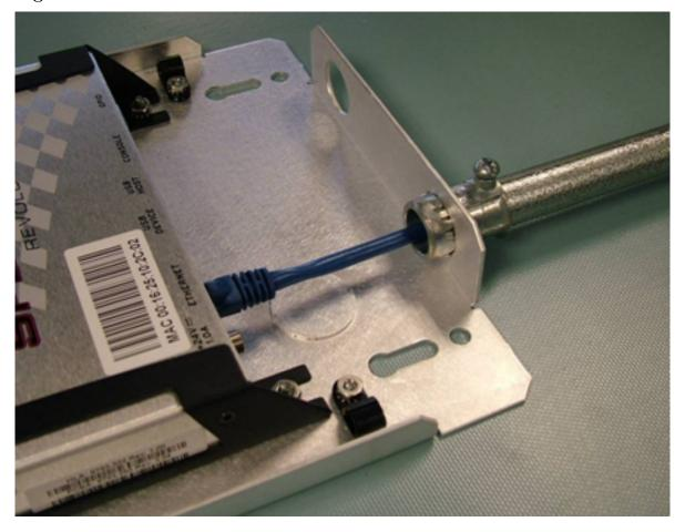
Figure C.5  $\frac{1}{2}$  inch conduit with a snap in flange connector
