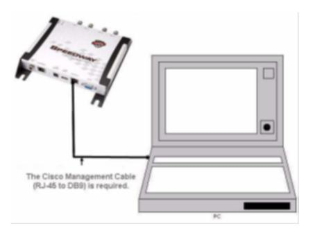
Figure 5.5 Speedway Serial Connection
