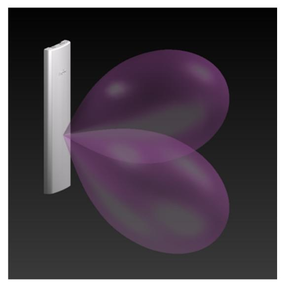
Figure C.1 xPortal Simulated RF Beam Patterns
