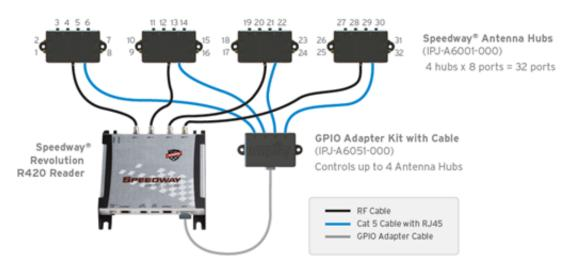
**Figure D.1** Speedway R420 Reader with four antenna hubs and GPIO adaptor for a total of 32 RF antenna ports.
