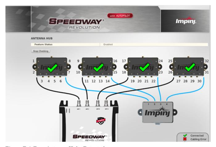
Figure D.3 Four Antenna Hubs Detected
