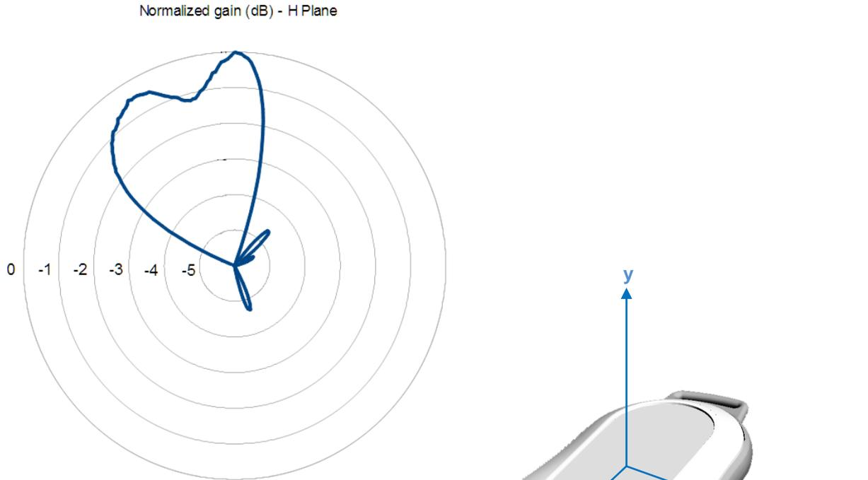
Fig. 10.3: qIDmini R1170IU Radiation pattern H plane
