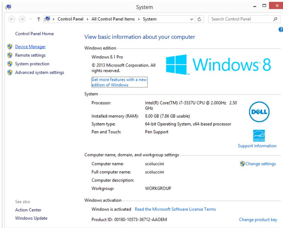
4. After having installed the driver, the reader is detected by the PC as an emulated serial port (VCP):
