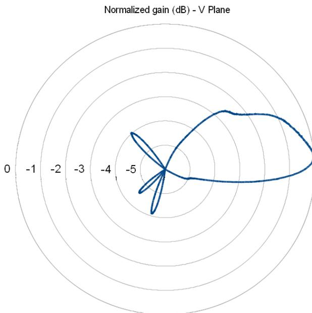
Fig. 10.2: qIDmini R1170IE Radiation pattern V plane
