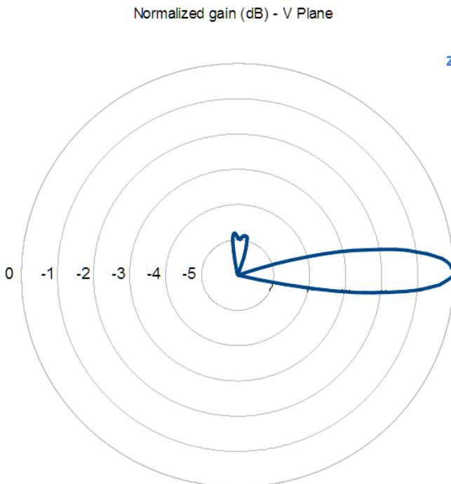
Fig. 10.4: qIDmini R1170IU Radiation pattern V plane
