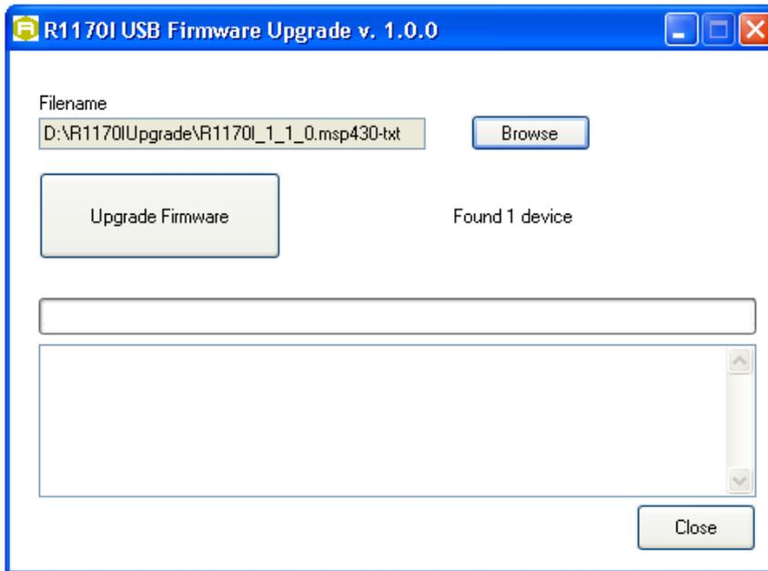
7. Click on the "Upgrade Firmware" button and wait for the upgrade process to be completed.
