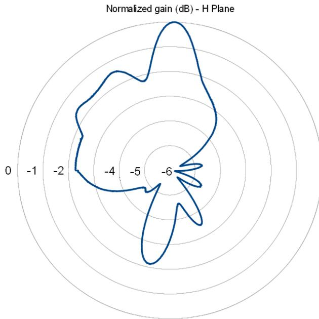
Fig. 10.1: qIDmini R1170IE Radiation pattern H plane
