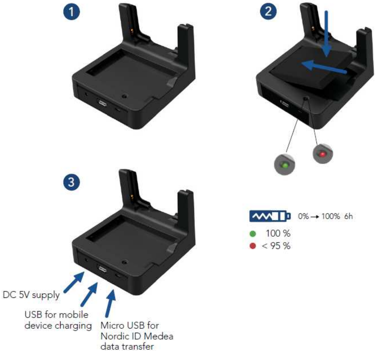
Picture 5 Battery charging in desktop charger
