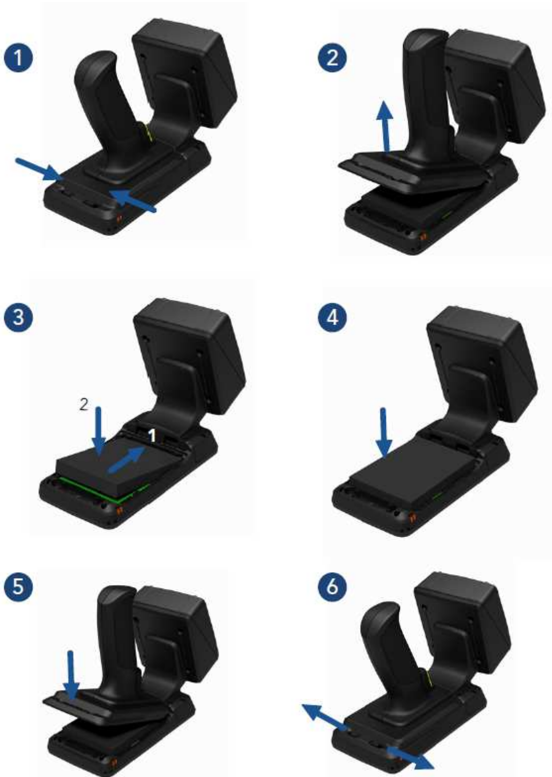
Picture 2 Installing battery
