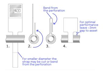
Ideal installation conditions are +20°C (+68°F) / 50% RH. For exceptional conditions, please contact Beontag. Bond strength can be improved with firm application pressure. Minimum bending diameter of the **Beontag LoopTag** is defined to be 50mm, excluding the strap part. Never touch on the location of the IC. Tag polarization should be taken into account in case liner polarized reader antennas are used.
